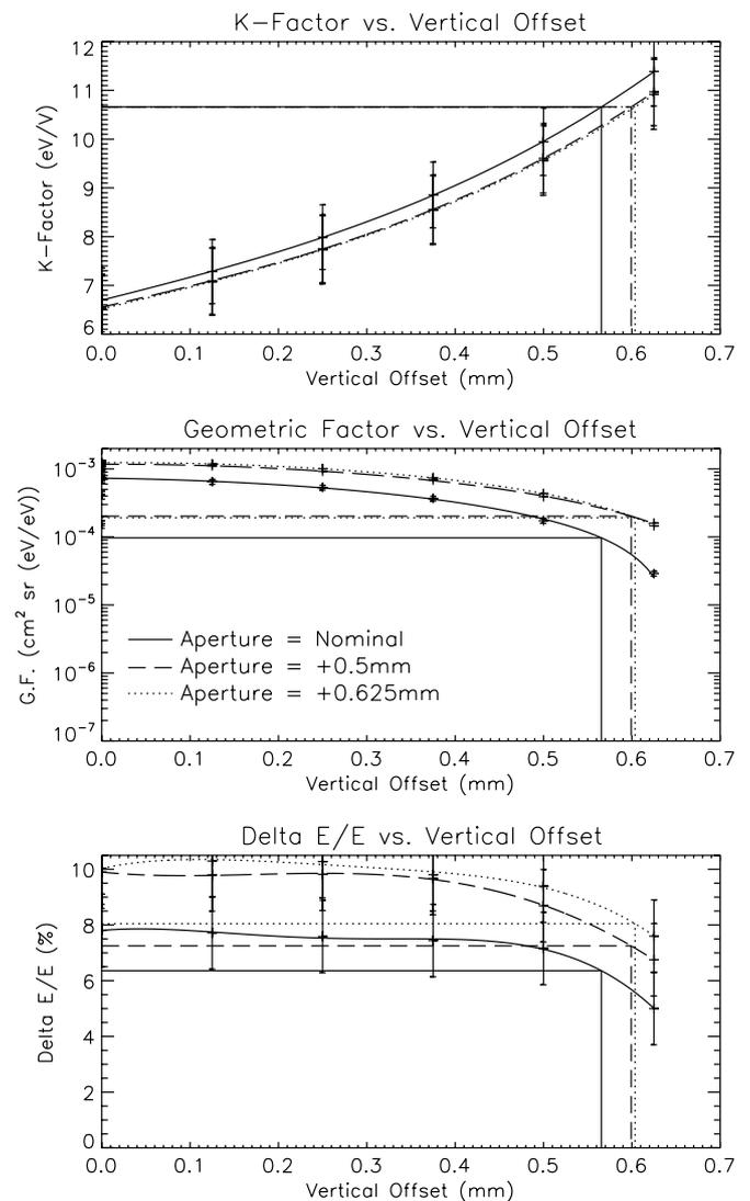
Figure 4. The effect of a vertical offset of the inner hemisphere on G.F.,  $K$  and  $\frac{\Delta E}{E_0}$ .
