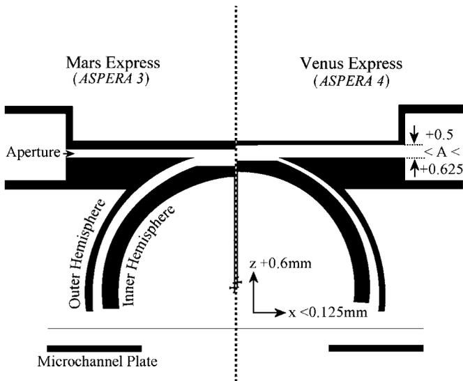
**Figure 1.** Cross section of ASPERA-ELS (to scale), showing MEX (left) and VEX (right), according to this study.
