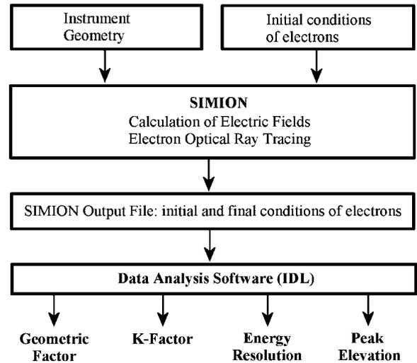
Figure 2. Flowchart showing the simulation method.
