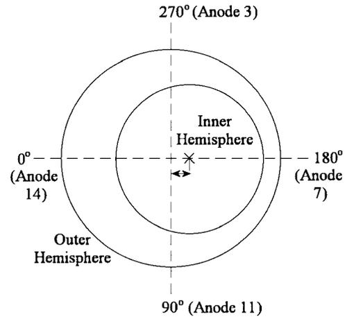
Figure 3. Schematic showing the four simulated lateral misalignments (offset greatly exaggerated).
