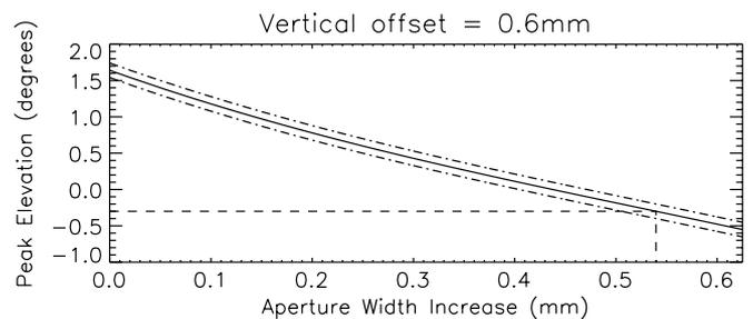
**Figure 6.** Peak elevation versus increase in aperture width, at an interpolated inner hemisphere vertical offset of +0.6 mm.
